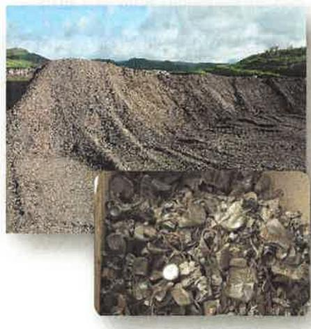
FIGURA 2: ESCÓRIAS INERTES (EM CIMA) E ESCÓRIAS FERROSAS (EM BAIXO)
